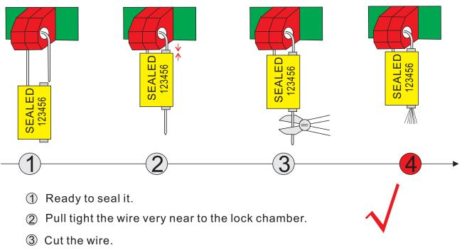
Because it is NPC wire, after cutting the wire, The wire scatter by itself.
